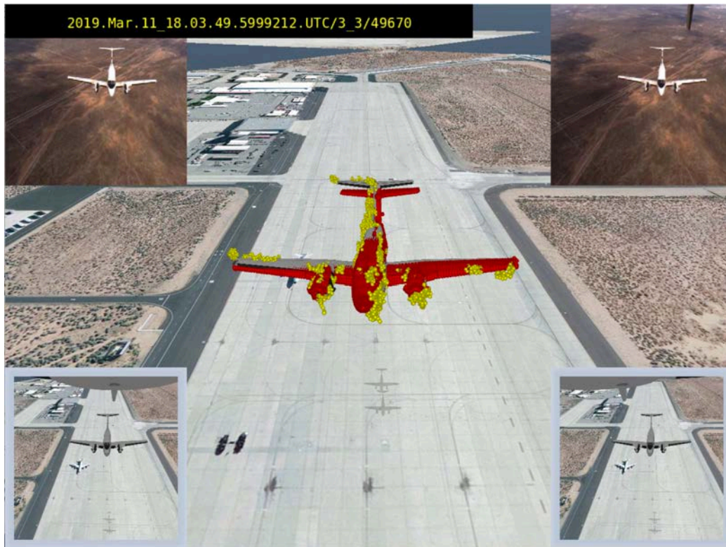
Figure 27: A Sample Relative Pose Estimation for Flight 3.3 Corrected for Camera Calibrations and Initial Hardware Errors
