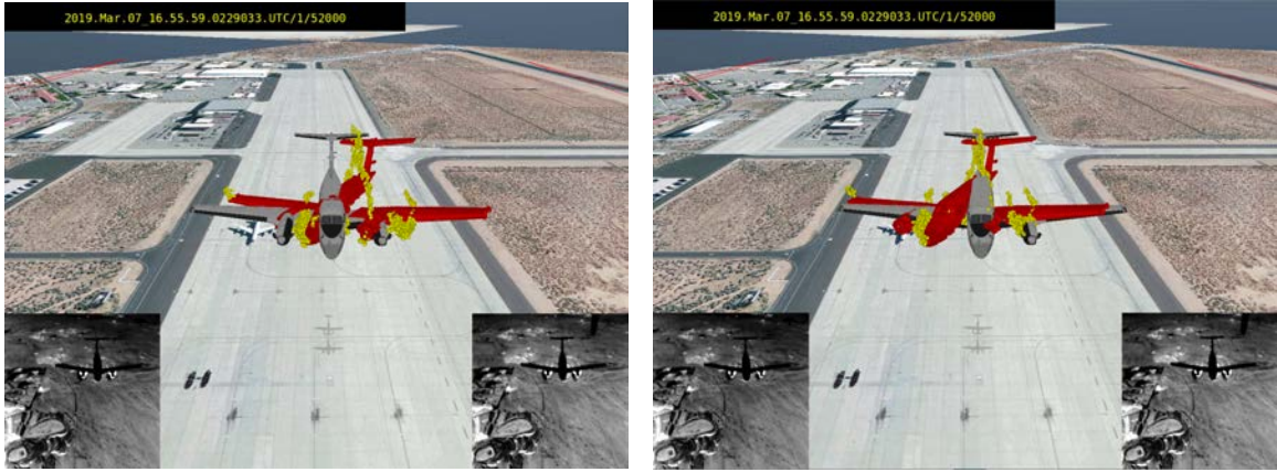
(a) Initial Optical Center Calibrations Illustrated Initial Sensed Red Model Placement (b) Modified Optical Center Calibrations Illustrating Altered Sensed Red Model Placement
