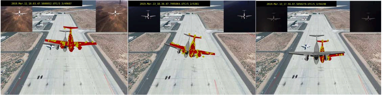
Figure 13: A Set of Relative Pose Estimations Using Original Calibrations Without Correcting for Errors
